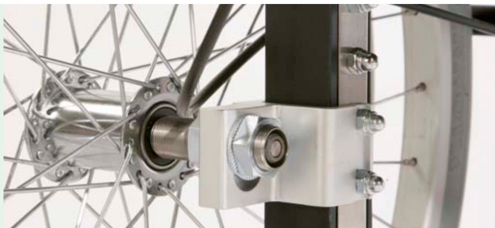
Rear wheels with quick-release axles
