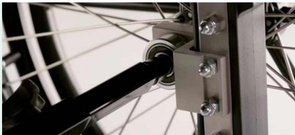
One-arm drive with telescoping axle for independent mobility
