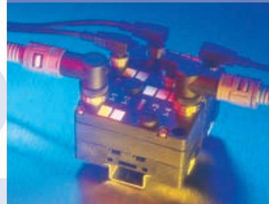
We provide our hydraulic balers with an AS interface (AS-I bus) to ensure better control of our machines. This AS interface is used to read the data collected by the sensors during the production process.
