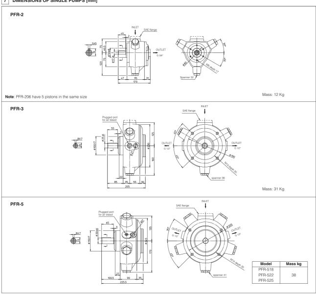
(ullet) SAE flanges are supplied with the pump
