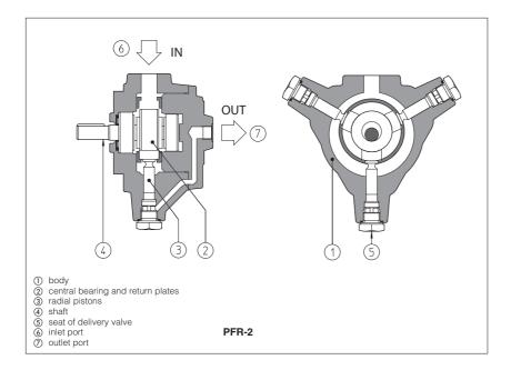
PFR are fixed displacement radial piston pumps with positive drive construction of the pistons (3) (without return spring) for high performance and low noise level.
