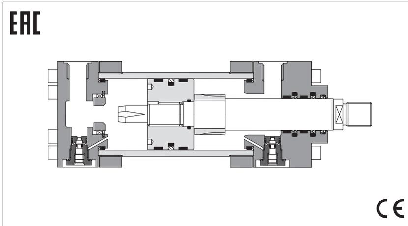
CN cylinders have engineered double acting construction, designed to suit the requirements of industrial applications: top reliability, high performances and long working life.
