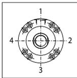
FRONT HEAD: **B1** = oil port position; **E\*** = cushioning adjustment position
