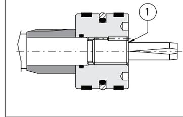
The rod and piston are mechanically coupled by a threaded connection in which the thread on the rod is at least equal to the external thread KK, indicated in the table [7]. The piston is screwed to the rod by a prefixed tightening torque in order to improve the fatigue resistance. The stop pin ① avoids the piston unscrewing.
