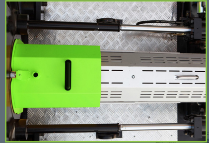
Two carriage pistons – ensures reliable operation over an extended working life
