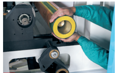
D Install new sleeve and assemble in the pre-printing position.
