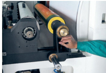
A Unlock the side handle in the air mandrel in order to change the sleeve.
