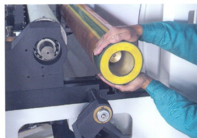
D Install new sleeve and assemble in the pre-printing position.
