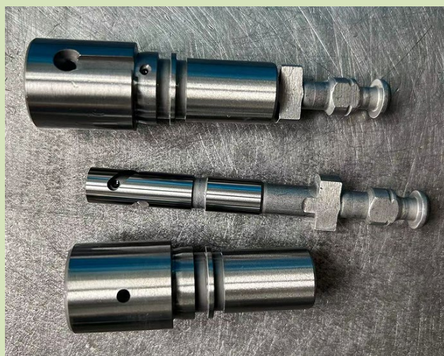
33-01,U5015,d=9mm ( end-milling groove by CNC)
