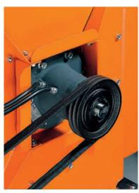
For the suspension of the impellers, quality components are exclusively used which are more than able to cope with the loads involved in fan construction. This results in the particular wear resistance and very long lives of Schuko fans.
