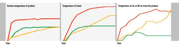
Tests performed at an ambient temperature of  $22 \,^{\circ}\text{C} + -2 \,^{\circ}\text{C}$  compare the HELISEA 110 towel-warmer heater (RED LINE) with towel-warmer radiators featuring an equivalent electrical input and size but based on traditional heating technologies: products with internal fluid circulation (YELLOW LINE); products with a standard heating element (GREEN LINE).
