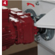
Robust engineering drive. Two strong gear motors drive the primary crusher's cutter shafts.
