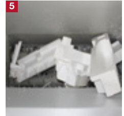
An efficient primary crusher with two cutting blade shafts crushes the parts into 20-50 mm sized small pieces.
