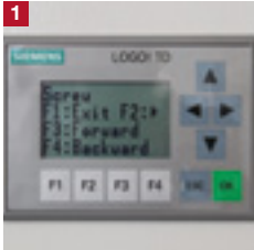
Operating display panel with function keys. Seven application programs can be adapted, as required, to a wide range of materials.
