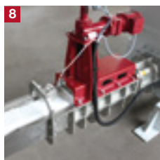
The fully automatic pressure regulator (ADC) with lifting spindle technology (no hydraulics or pneumatics) enables the production of highly compressed blocks.
