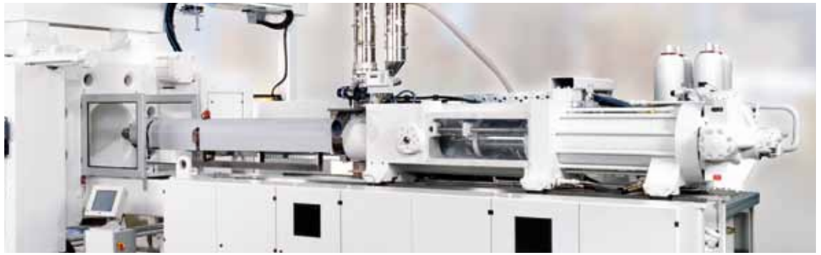
Hydraulic direct screw drive for highest repeatability and quality
