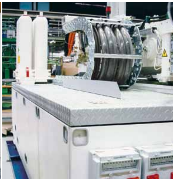
Encapsulated hydraulic drive, soundproof housing
