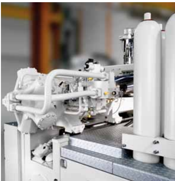
Control valves close to consumers for a highly consistent and stable process.
