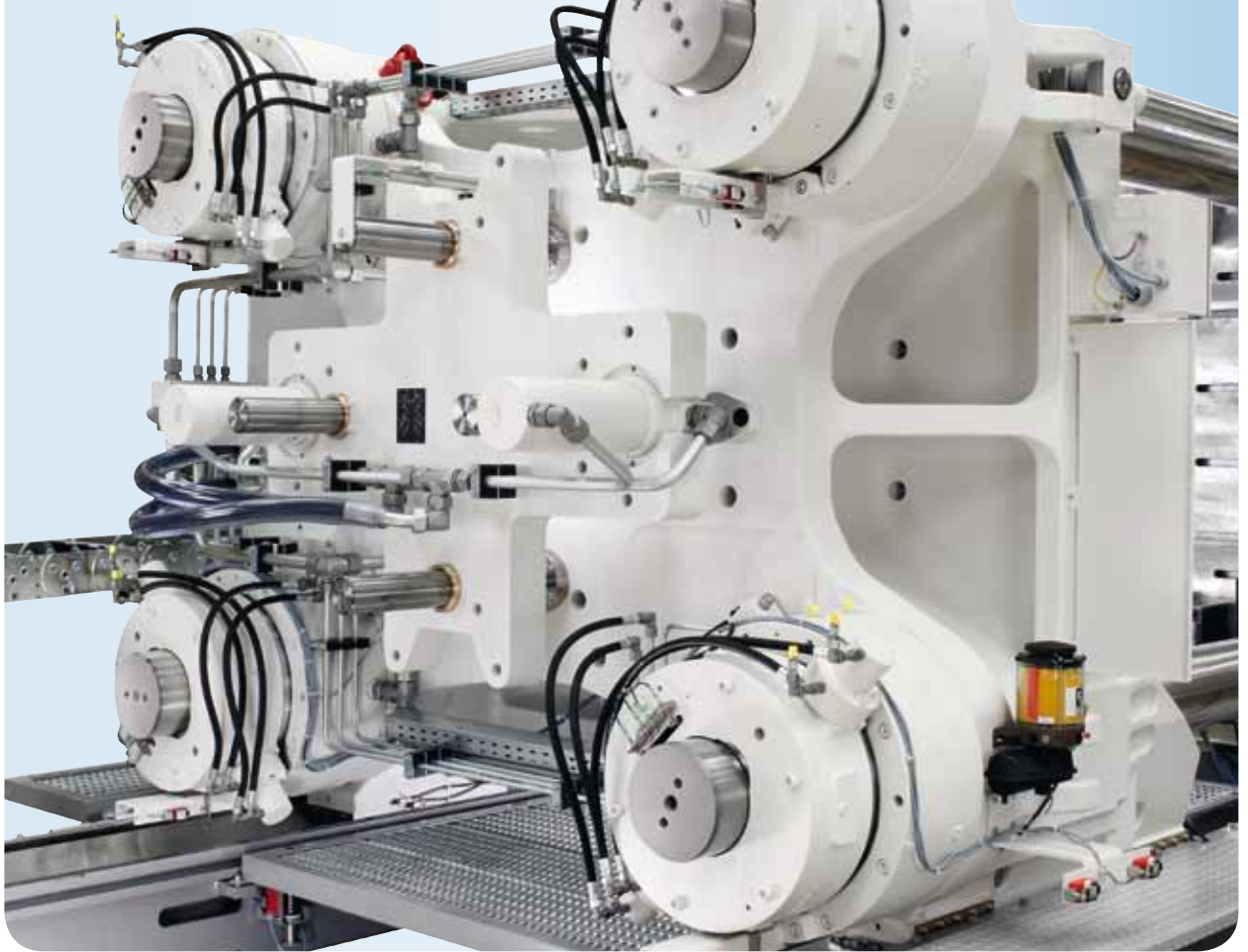
Moving platen as a rugged, FEM-optimized box structure
