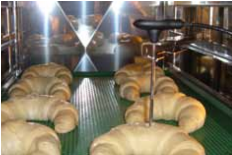
Croissants rise quickly, so insert the CT probe vertically. Use the positioning aid.
