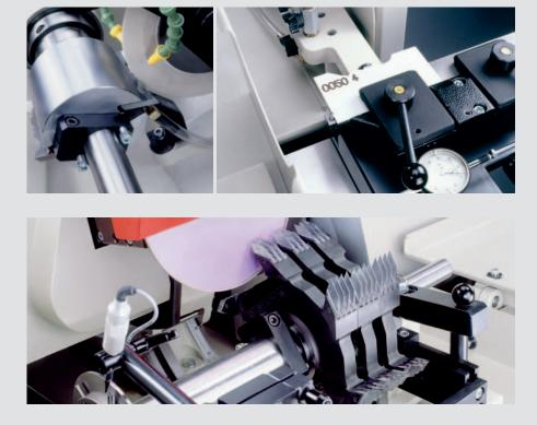
**Profile ground knives** are shaped and resharpened to a profile template on the back of the knife. This ensures absolute profile precision and optimum cutting angles for all types of species and materials. Sharp tools, perfectly ground for precision running.
