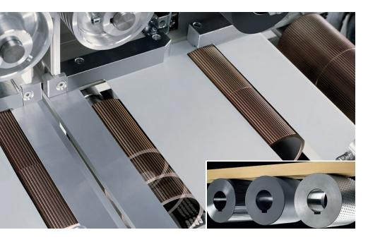
Different wood qualities impose different requirements. Thus, the feed rollers of the OptiCut 200 II can be changed very quickly in order to respond to the respective requirements. Rough and planed qualities can now be readily processed in the same shift, and resincoated rollers are easily cleaned for consistently high performance in every shift.
