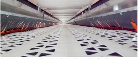
Central, 500 mm wide longitudinal egg belt with triangular holes for a stable position of the eggs
