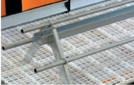
A-frame 3000 with three perches and one feed line
