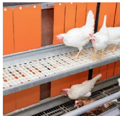
The tilting floor closes the nest after the laying period
