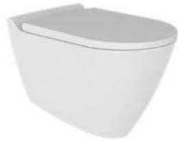
KINOA NO-RIM SUSPENDED TOILET MNKA052N1VP1W3QA0 (Concealed Mount) 520x345 mm Bidet tube, special metal mounting adapter, spiral hose included. Concealed cistern and toilet seat are not included. White
