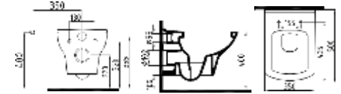
PIAZZA SUSPENDED TOILET 500 mm DRKA050AMVP1W5QA0 (Open Installation) 500 mm bidet pipe, spiral hose included.
