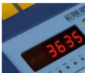
RED LED DISPLAY for a clear display of the total weight.
