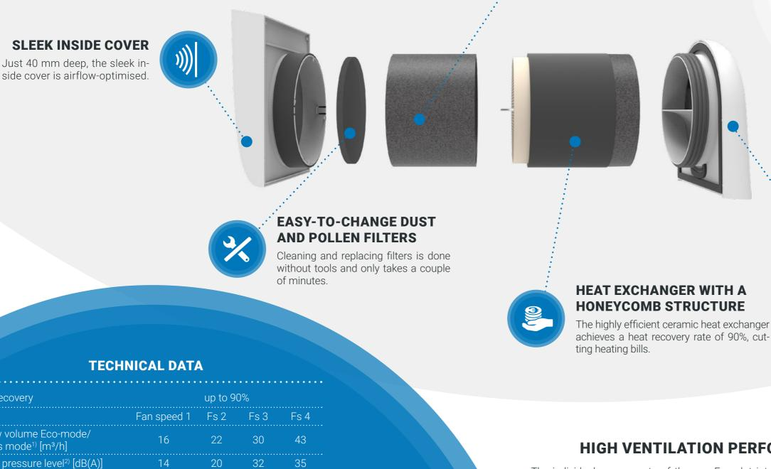
The individual components of the easyFan slot into the 160mm-diameter installation cylinder one after another. Installation requires no tools - just slot in the components. Ultra-compact and quiet, they offer top performance. The individual components of the easyFan slot into the 160mm-diameter installation cylinder one after another. Installation requires no tools - just slot in the components. Ultra-compact and quiet, they offer top performance.
