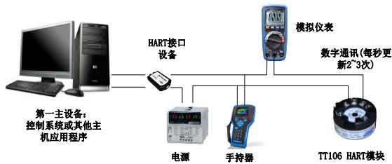
Figure 3.1 4~20mA compatible mode
