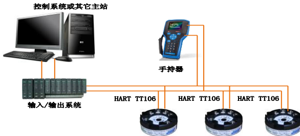
Figure 3.2 HART Networking mode
