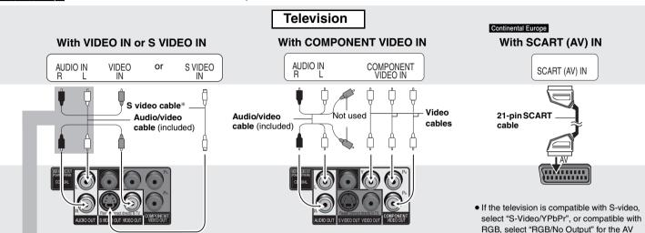
You can connect the audio cable to the 2channel audio input terminals of an analog amplifier or system component to enjoy stereo sound.
