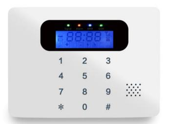
Input \*+phone number+# on the key board, the host will dial out immediately. For example, if you want to call the number 1381111111, dial "\*1381111111# "directly on the keyboard.
