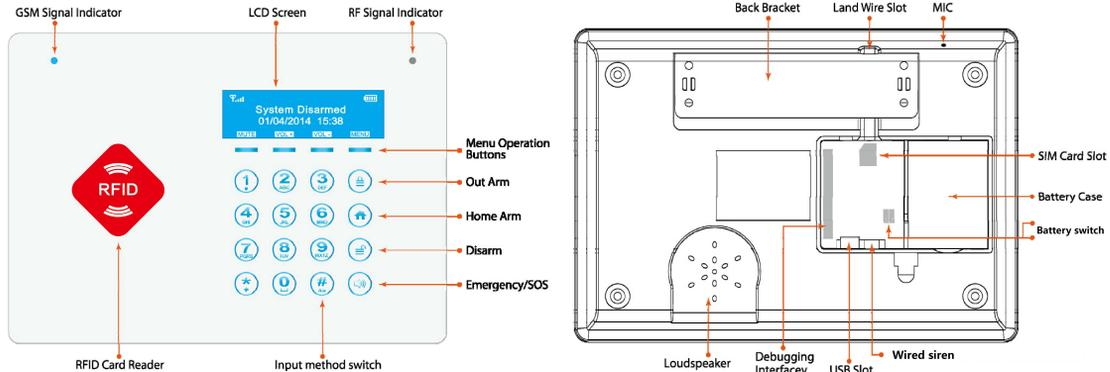
**【GSM Signal Indicator】:** No SIM card or searching network: flashes once per second ;GSM Signal in normal: Flashes once per 3 seconds
