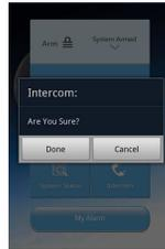
②call the system host by phone and input the password as the voice prompt. The default password is 888888. Press key “4” to make the intercom.
