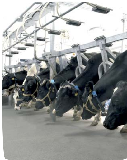
Proactive front barrier during indexing
