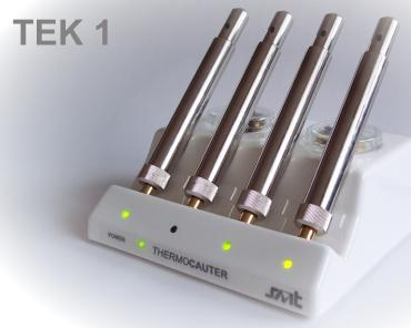
The pencil thermocauters are designed for ambulatory surgical use, primarily in dermatology where they are used to remove small, varicose growths, papilomas, warts etc. The basic principle of the thermosurgery is an excision of these growths by burning their stem and/or a coagulation with a hot wire loop.
