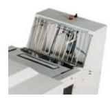
This simple stacker aloow to collect collar and cuffs after fusing, this system will be perfect also without cooling system because the parts will have their time to cool on the stacker skid.
