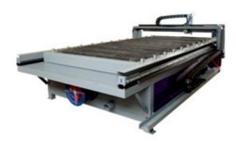
Legend III could support the steel plate with heavy weight. Since the cutting table is higher than the longitudinal guide, it is very convenient to load and unload the steel plate.
