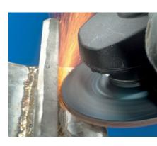
Soft general-purpose tool of hardness M, with aggressive grinding performance and long tool life
