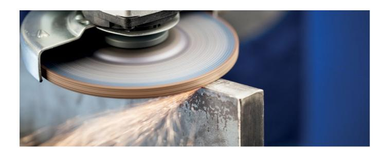
Very soft special tool of hardness H, with exceptionally aggressive grinding performance. Operates without tool clogging even on soft, lubricating aluminium
