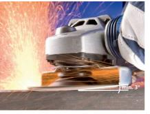
Integrated glass fibre backing pad for hard and tough use, and for work on edges.
