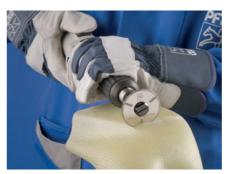
Accessories for mounting diamond cut-off wheels up to a diameter of 75 mm.
