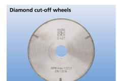
Electroplated diamond cut-off wheels are characterized by their particularly efficient cutting performance because of their large chip spaces. They are used with grit sizes from D 64 to D 427 for cutting hard materials such as tungsten carbide or ceramics and fibrereinforced plastics (GRP/CRP).
