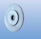
For mounting flap wheels and POLINOX® grinding wheels on drive spindles. The centre hole of the flange can be drilled out according to the dimension of the given drive spindle. The clamping flanges are designed to lie countersunk in the tool.
