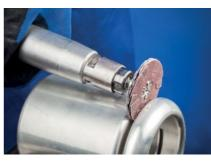
Reduces setup times significantly. The overlap slotted discs can be changed without removing the arbor from the collet mounted in the tool drive.
