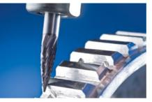
Pointed tree-shaped burr according to DIN 8032 with cut conforming to DIN 8033, flattened tip.
