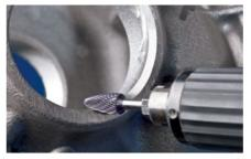
Tree-shaped burr with radius end according to DIN 8032 with cut conforming to DIN 8033.
