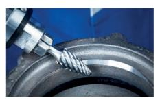
Tree-shaped burr with radius end according to DIN 8032.
