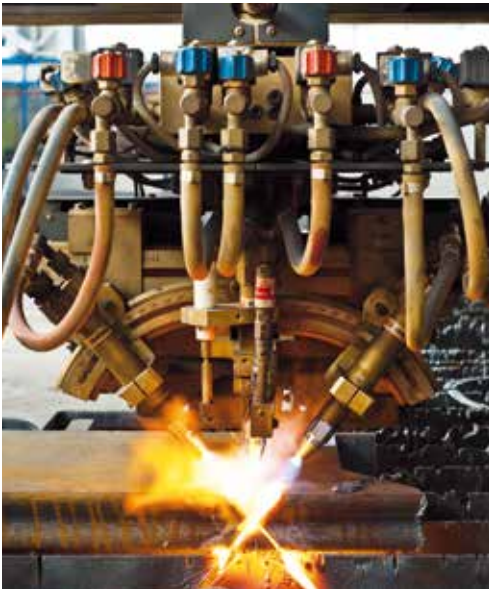
Testa bevel 3 cannelli oxy • 3 torches oxy head
