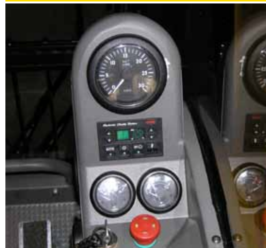
Instrumentation VDO oil level and water temperature sensors, self diagnostics
