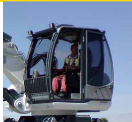
Cab with windows that open on three sides for maximum comfort
