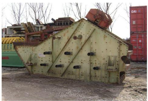
This High Capacity Feeder Screens might feeds about a 150 t/hr. to gravel aggregate washing & screening plant.
