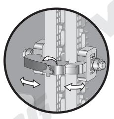
Turn the knob counterclockwise, Move the curvature adjustment piece to the sides or in the middle. Move to the sides, the screen surface will be the inner arc; to the middle, the screen surface will be the the outer arc. When adjust the proper angle, tighten knob clockwise, then radian is fixed well.
